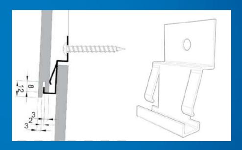
MEG FIXING SYSTEMS | Invisible fixing with profiled edged panels in horizontal running aluminium hook profile
