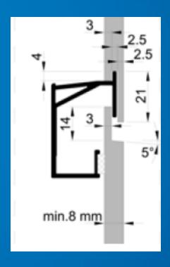
MEG FIXING SYSTEMS | Invisible fixing with profiled edged panels ir horizontal running aluminium hook profile
